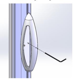
Step 2. Using #6 x 1/2" self-drilling screw, anchor the handle in position through the clearance hole in the handle.
