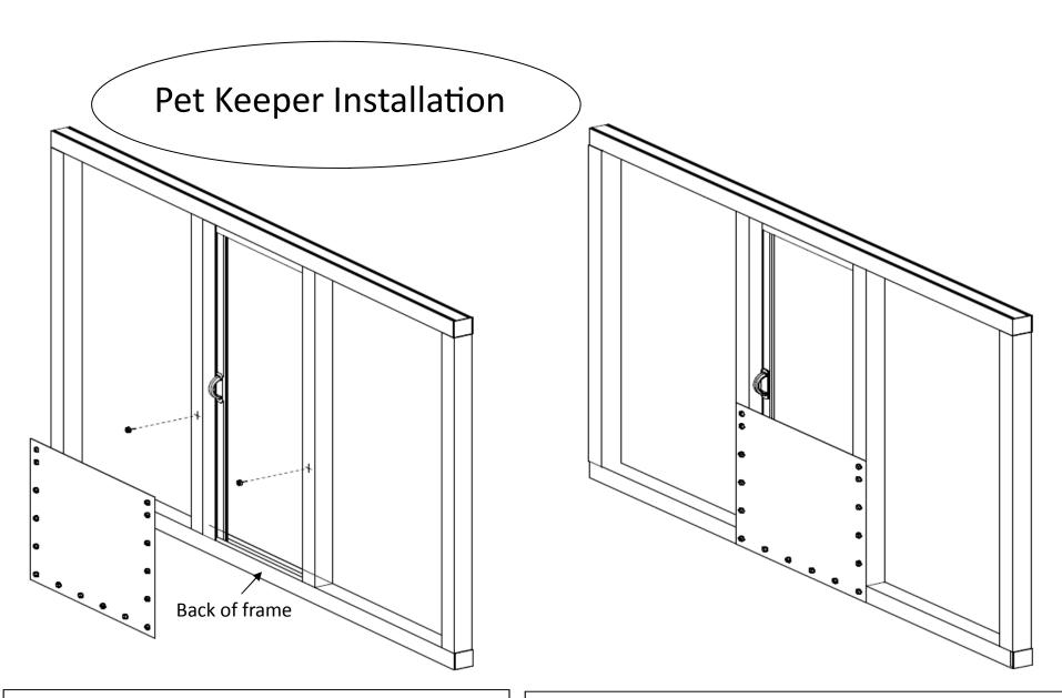
1. Measure up 33-1/8" from the bottom of frame and place a mark centered on vertical members. Screw in male portion of snaps using #2 phillips driver.
