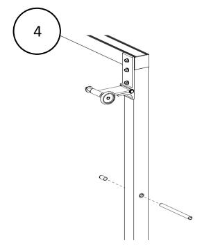
Drill marked location using 1/2 " drill bit and insert plastic bushings with larger flanged side of bushing facing outward.
